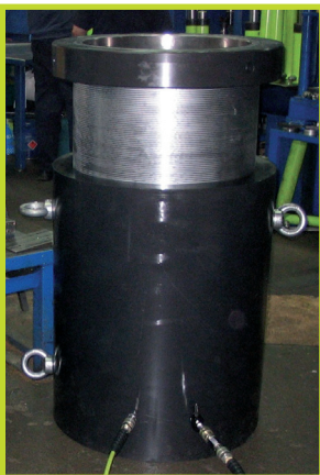
Double acting cylinder with lock nut. 1.500 Tn capacity and 500 mm stroke.
