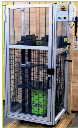
140 Tn capacity and 250 mm stroke press with special protection.
