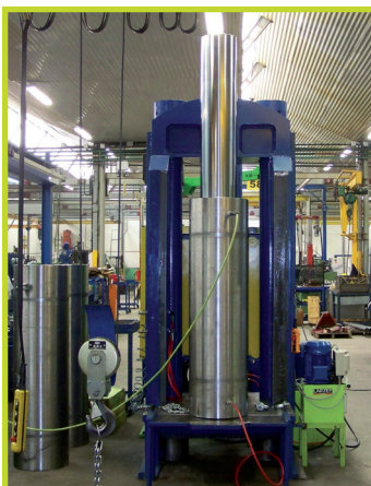
Double acting cylinder with 1.250 mm stroke.
