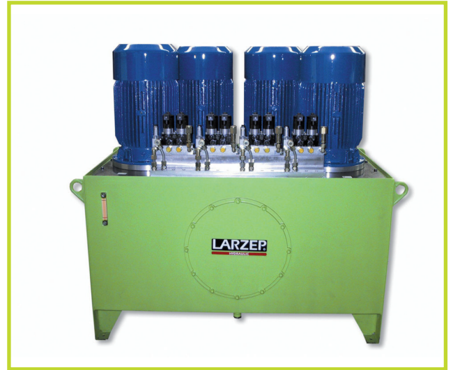
Hydraulic powerpack, 600 litres capacity, with 4 pumps and 4 exits each. Each pump is connected to the 4 solenoid valves.
