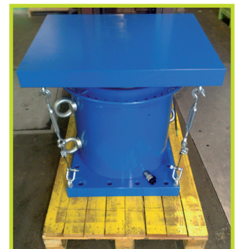
1.000 Tn single acting cylinder with lock nut and tilting saddle. Supports a 12% side load.
