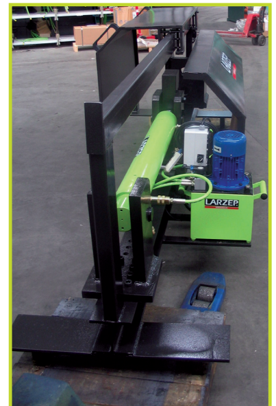
Wheel crusher. 23Tn capacity and 800 mm stroke.
