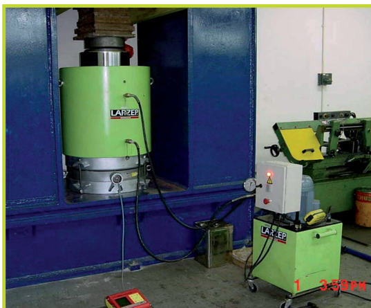
Heavy duty press, 1.500 Tn capacity and 150 mm stroke press with 50 litres powerpack with solenoid control.
