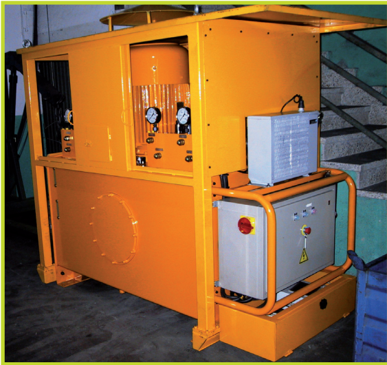
Synchronized Lifting system, 1.000 litres oil capacity. With 2 synchronized outlets + 2 manual outlets. Flow 25.5 l/min.
