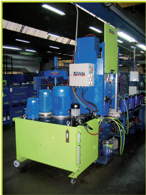
Hydraulic powerpack, 600 litres capacity with 3 different pumps to work at different pressures and flows.
