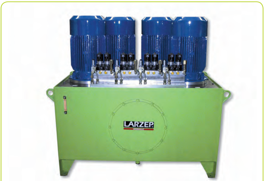
Hydraulic powerpack, 600 litre capacity, with 4 pumps and 4 exits each. Each pump is connected to the 4 solenoid valves.
