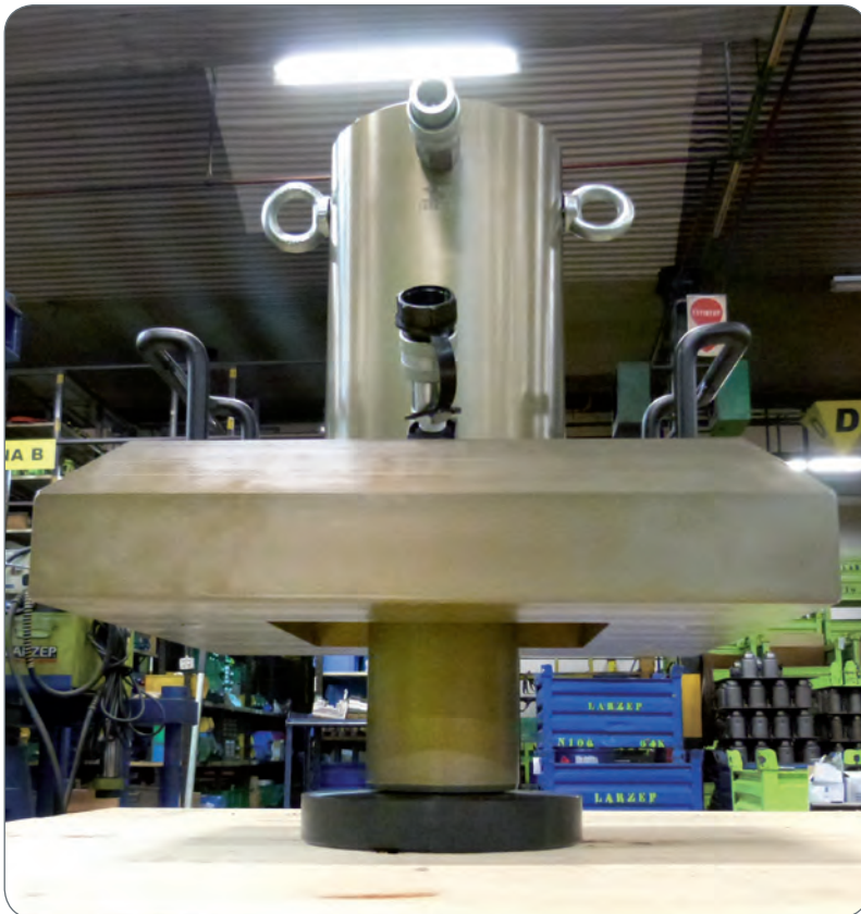
Step by step aluminium cylinders. Stage lifting.
