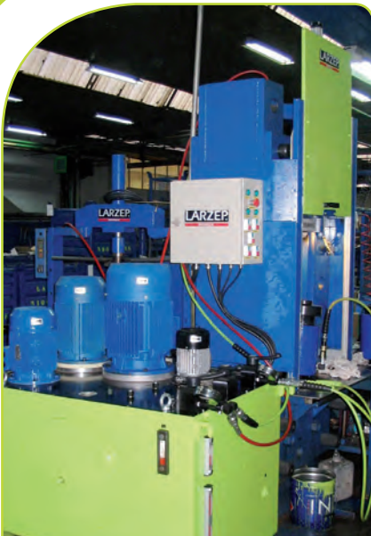
Hydraulic powerpack, 600 litre capacity with 3 different pumps to work at different pressures and flows.
