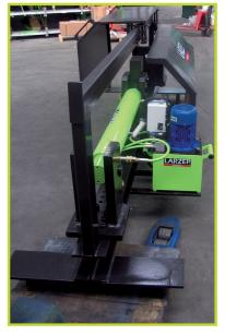
Wheel crusher. 23Tn capacity and 800 mm stroke.
