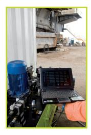
The control point for the jacking system was a laptop computer, easy to use, allowing jacking accuracies of multiple cylinders to within 1 mm.
