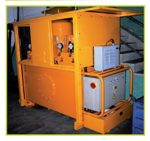
Synchronized Lifting system, 1.000 litres oil capacity. With 2 synchonized outlets + 2 manual outlets. Flow 25.5 l/min.
