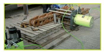
Double acting cylinders D35030, 350 ton and 300 mm stroke were used together with a HAM7645 110 volt 2.1 litre per minute power pack with remote control pendant for safety and ease operation.
