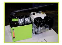
10 litres Petrol powerpack with manual pump, 2 valves and by-pass.
