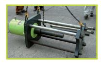
The pin was pushed through; in this case it took 251 metric tonnes to break the grip of the pin which was very badly worn.
