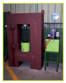
30 Tn capacity and 90 mm stroke press with 50 litres powerpack with 4 ways.
