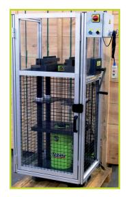
140 Tn capacity and 250 mm stroke press with special protection.
