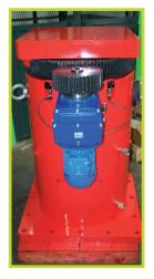
Double acting cylinder with lock nut and gear wheel.
