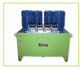
Hydraulic powerpack, 600 litres capacity, with 4 pumps and 4 exits each. Each pump is conected to the 4 solenoid valves.
