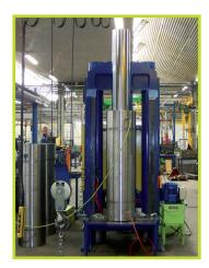
Double acting cylinder with 1.250 mm stroke.
